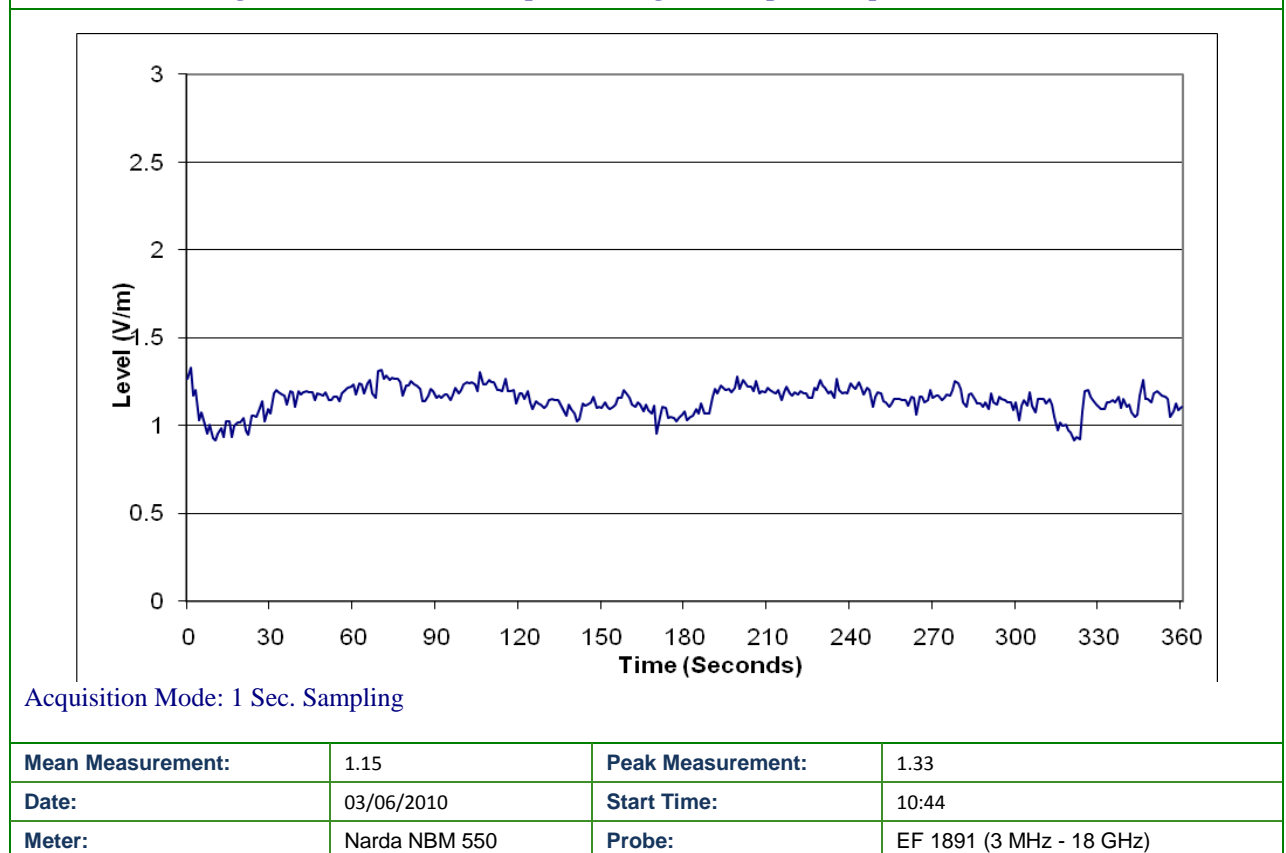
Electric field strengths recorded over 6 min period using 18 GHz probe at point of max NIR:
